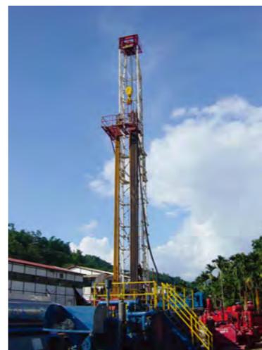
Model: BR. 5000R, made in Australia. Max dig depth: 2000m, suit for hot spring well, water well, gas well and mining industry exploration.
