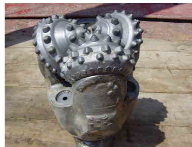
Imported tungsten carbide steel bit Function: To increase the drilling power
