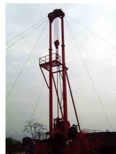
Model: Sullivan, made in S. Africa Max dig depth: 3000m, suit for hot spring well, water well, gas well, oil well and mining industry exploration.
